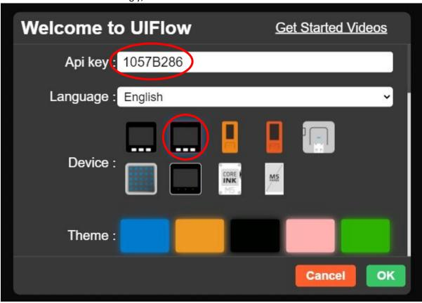
Notice that, the red device (M5Fire) is selected, this must be chosen for the software to work correctly.
