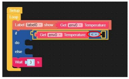
In the block programming menu, select Math, drag the number block and snap in the last slot in the comparison block.
