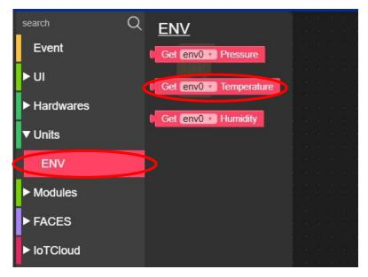
You can see the 3 data types captured by ENV sensor. We will read and display the temperature first.
