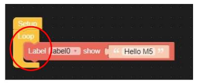
Under the block programming menu, click on Units and then click on ENV. Drag the Get Temperature block and snap it inside the Label block, replacing "Hello M5".
