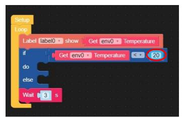
We now need to tell the M5Stack that if the temperature is less than 20, we flash a blue light on the M5.
