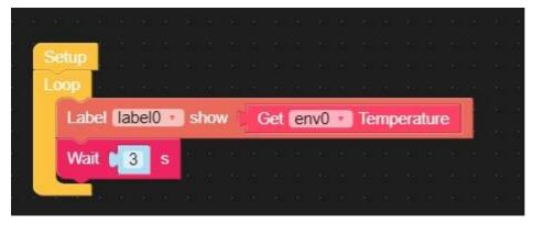
We will add conditions to get the M5 to flash red if the temperature is equal or greater than 20 C, and flash blue if the temperature is less than 20 C.
