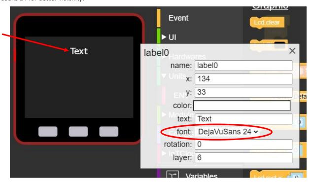
Under the block programming menu, click on UI and then click on Label. Drag the first Label block and attach it in the middle of the Loop block. When dragging, it will look a greyish colour, it will change back to its bright pink colour when it is attached to the loop.
