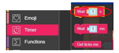
Click on Timer and drag the Wait block and snap it under the Label block. Make the wait time 3 seconds.
